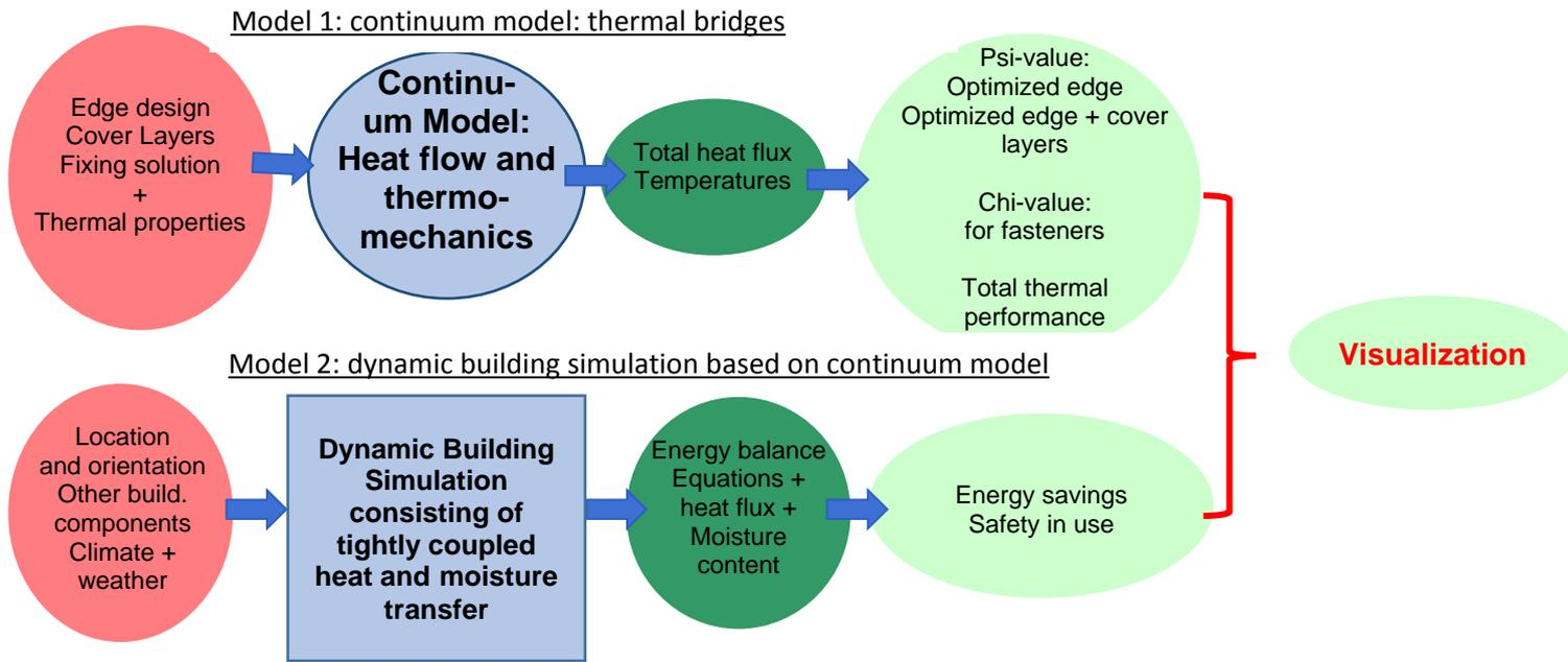
First the components are modelled as a static situation. The heatfluxes will be used to optimise the design. For this optimised design a dynamic building simulation will be done. The building will be modelled in a dynamic situation to catch transient behaviour;
