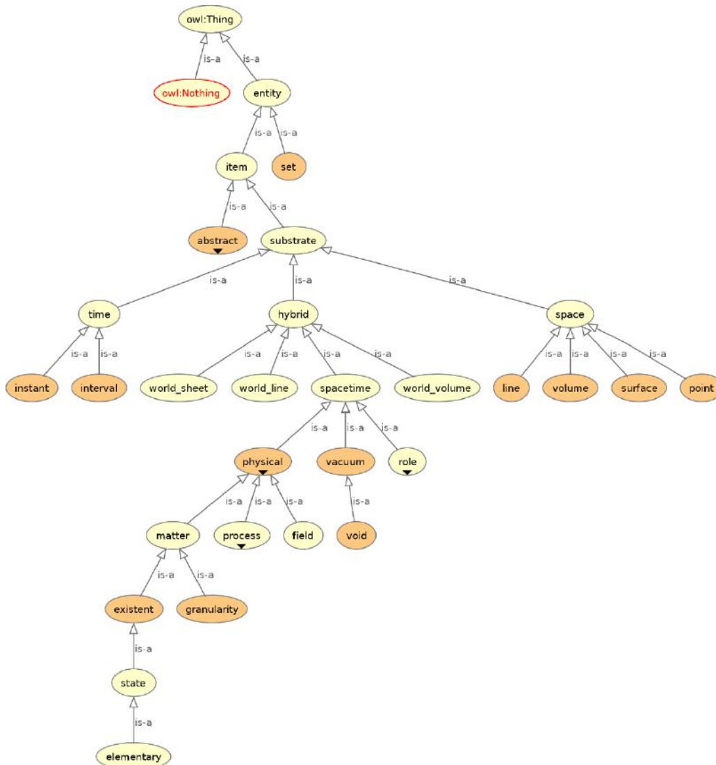
Figure 1 – The base branch of EMMO showing the elementary that constitutes all matter. All real materials will be defined in the state branch while natural laws, models and properties will be defined in the abstract branch.
