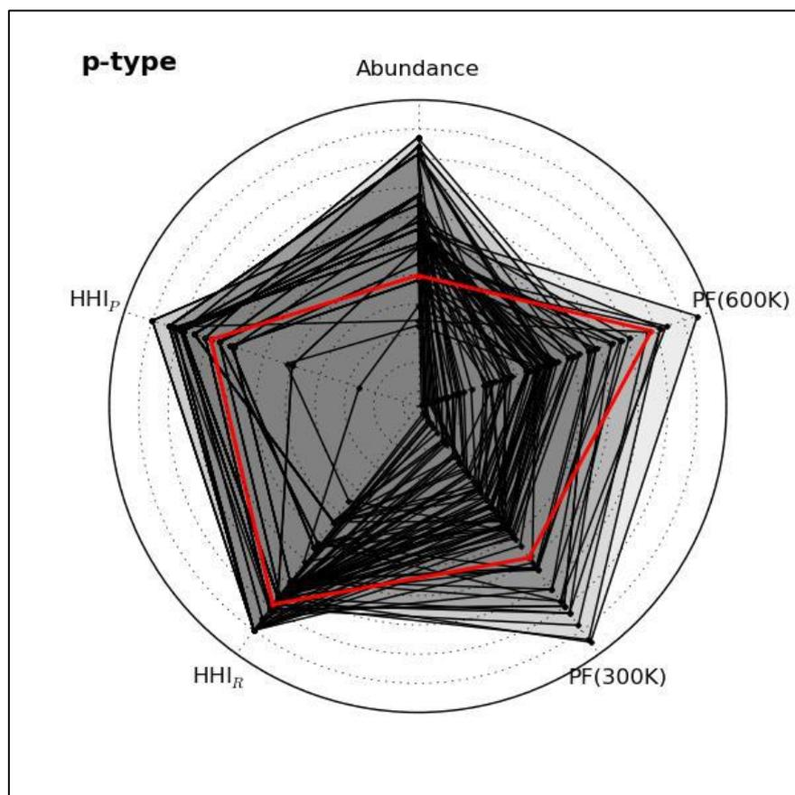
*Radar plot of the abundance, supply risk (HHI<sub>production</sub> and HHI<sub>reserve</sub>) and calculated thermoelectric power factor PF for a range of binary sulfides. Each ring corresponds to one calculated semi-conducting phase. The red path corresponds to tin sulphide. (adapted from Reference [1])*
