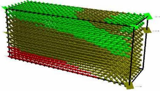
**Figure 3a.** A small volume interpolated using WinGeol based on just a few input points (represented by the square elements) – every Voxel contains orientation and rock type information (therefore the VOXEL is shown as a coloured arrow; level of confidence is calculated as well but not displayed here). This is used as an input for a further erosion / deposition simulation using SedTec. But can be already a valuable input by itself (e.g. for groundwater flow simulations).
