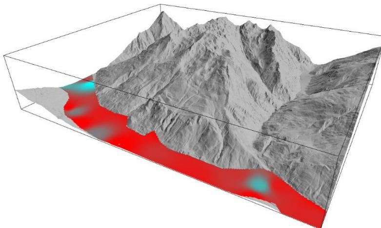
**Figure 1.** Negative effects of low density input data: Digital twin of a river, created with low density data sampling and standard interpolation techniques. Blue areas mark paleo river channel sediments and red areas other sediments.
