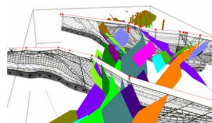
Especially difficult is the processing and interpretation of fault lines from heterogeneous datasets. Figure 4a shows lines representing faults digitized based on section images and Figure 4b displays some of these lines connected to fault planes. Faults are extremely important elements as they
