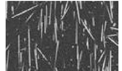
Short glass fiber reinforced thermoplastics (SFRT)
