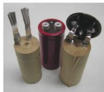
FIGURE 1. Aluminum electrolytic capacitors. The windings are composed of aluminum foils and cellulosic separators, and exhibit thermal anisotropy.
