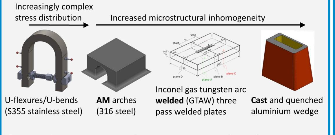
The samples are measured using neutron and synchrotron diffraction based techniques in addition to laboratory x-ray diffraction, (semi)destructive techniques and modelling.
