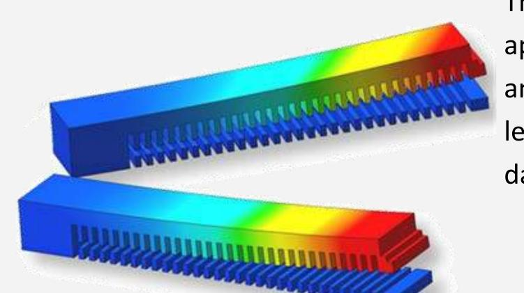
This requires the use of empirical approaches for heat source calibration and net impact of scanning at the macrolevel of simulation. Further experimental data is required to capture plasticity.
