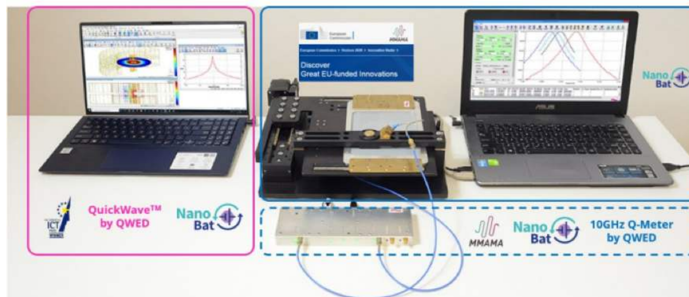
Implementation in the form of surface scanner for GHz-imaging of electronic and battery materials - Finalist of the European Innovation Radar Prize 2021.
