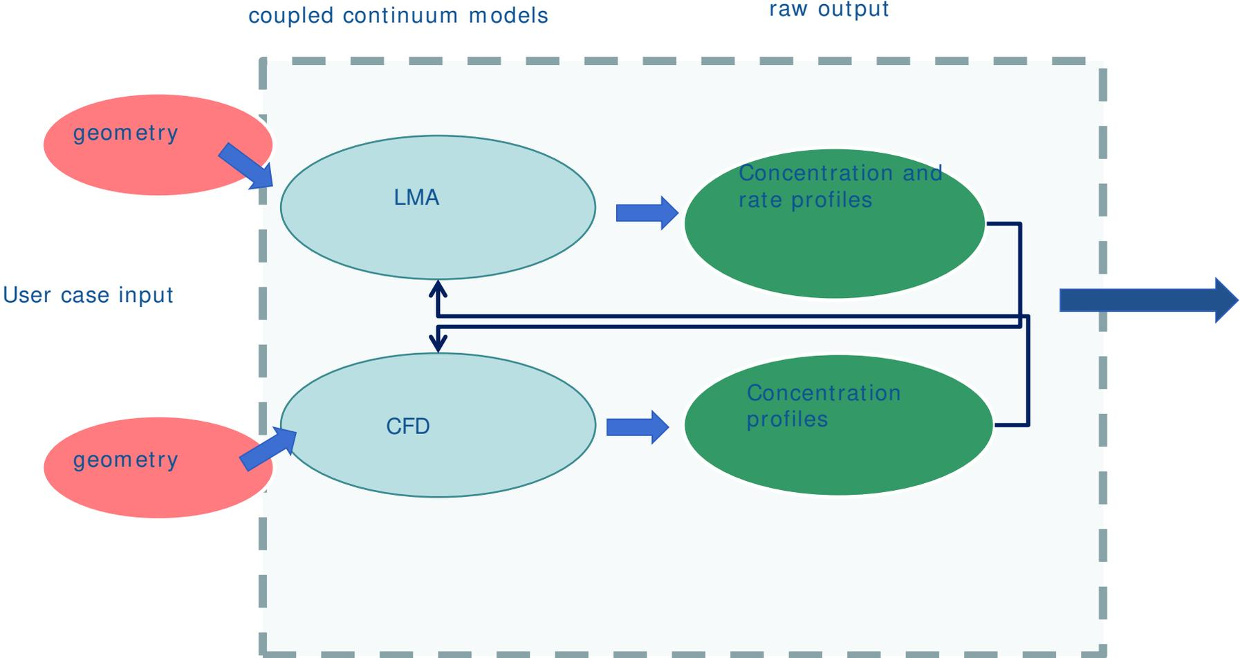
Details on workflow with coupled LMA and CFD models
